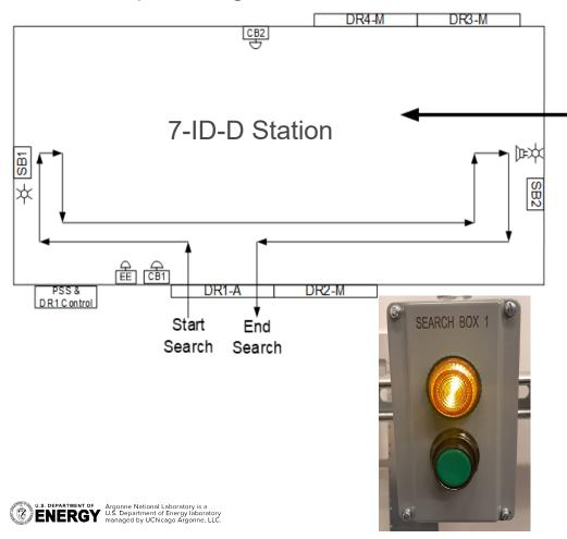
After completing the search, exit the hutch, go to the station panel and press and hold the "CLOSE" button.
